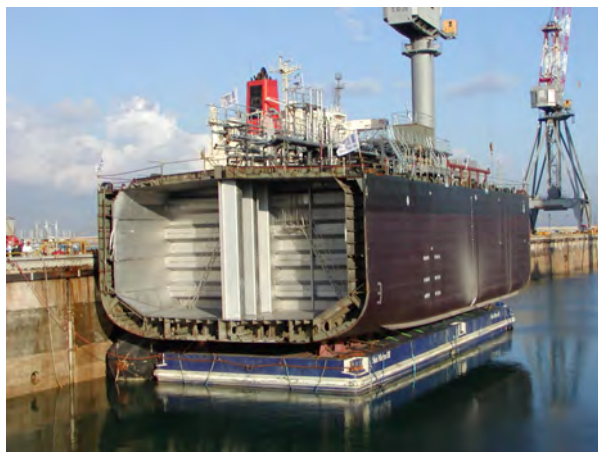
Figure 12.8. Cargo container made from 2205 in a parcel tanker
