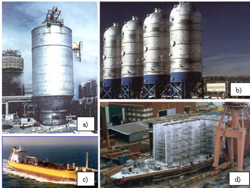
Figure 2.55. a) Paper pulp storage tank in New Zealand made of the S32304 duplex grade. b) Pulp and paper digesters in USA made of the S32205 duplex grade. c) A chemical tanker made of the S32205 duplex grade (La Tour Pomerol). d) A chemical tanker under construction made of the S32205 duplex grade
