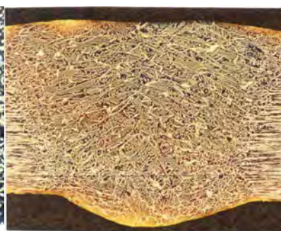
Figure 4.11. Microstructure of a plasma-welded SDSS SAF 2507 (thickness: 3 mm) [BON 94a]
