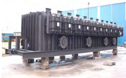
Figure 12.7. Series of evaporator shells in 2205 designed for an MSF plant
