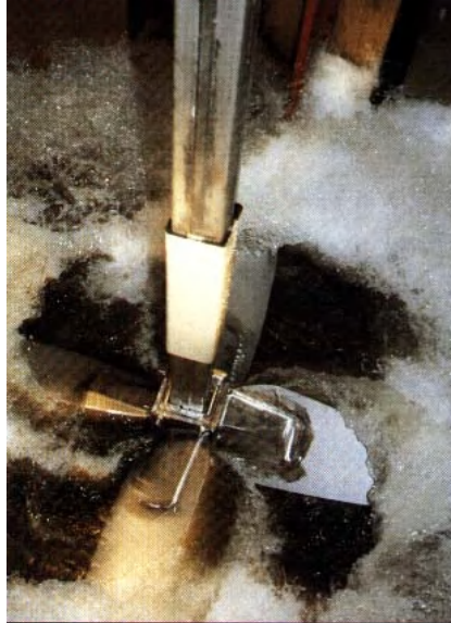
Figure 2.14. S32520 superduplex grade selected for an agitator working in an attack tank for phosphoric acid production (abrasion corrosion conditions)
